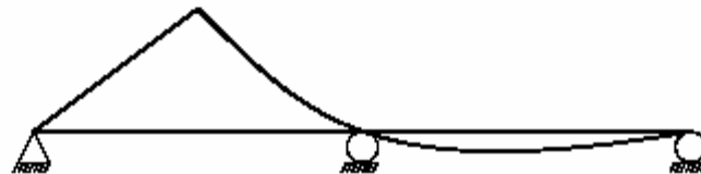
(b) Influence Line for Moment at Center of Left Span of Two Continuous Spans
