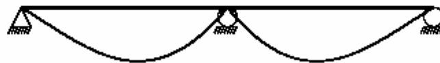
(c) Influence Line for Moment at Center Support of Two Continuous Spans
